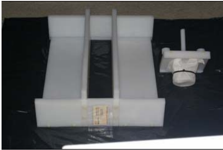
Figure 4: Device frame and weight with wipe with rod threaded through hole in slide.
